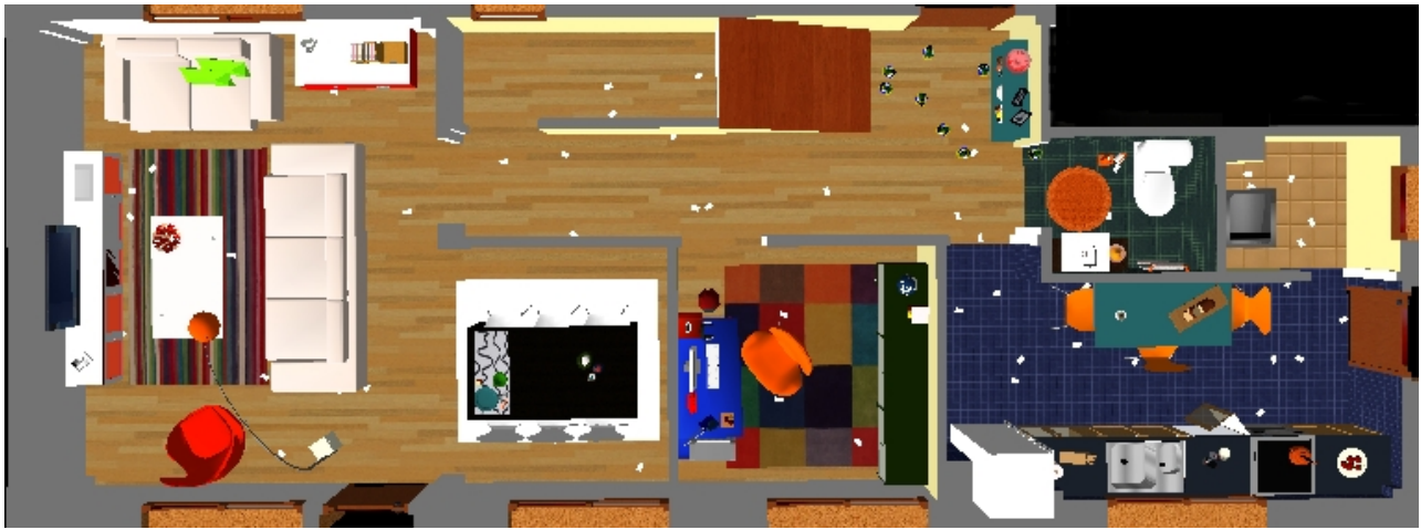
Fig. 2. Eight robots exploring the ground floor of a virtual home filled with 80 randomly distributed RFID cards.
